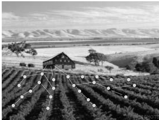
Figure 1-2: Possible deployment of ac-hoc wireless embedded network for precision agriculture. Sensors detect temperature, light levels and soil moisture at hundreds of points across a field and communicate their data over a multi-hop network for analysis.
