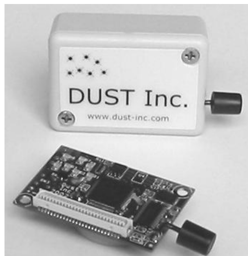
Figure 5-5: Follow-on to the Mica node, blue increase range and reduces power consumption. Blue nodes have a 4-6x longer battery life over Mica on alkaline batteries.
