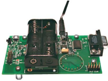
Figure 4-1. MICAz/MICA2 plugged into top-side of an MIB510.
